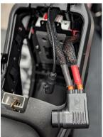
**Step 18:** Position the plastic trim behind the top tab of the controller and loosely install the (2) OEM bolts.
