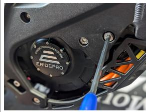
**Step 20:** Use the included (4) 6mm bolts and washers to install the side trim plates with a 4mm hex key. You can route the brake hose behind the trim plates.
