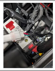
**Step 12:** Route the Positive and Negative battery harness wires down the back side of the battery support plate.
