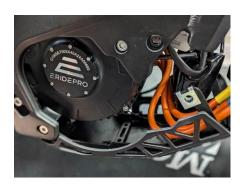
**Step 5:** Use a 5mm hex key to remove the (2) bolts in the upper portion of the frame. This allows you to hinge the battery support plate back to get better access to the breaker.
