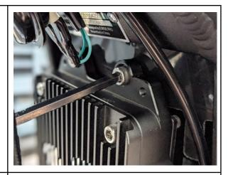
**Step 19:** Reinstall the (2) skid plate bolts with a 5mm hex key.
