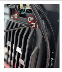
**Step 2:** Use a 4mm hex key to remove the lower controller bolts. Use a 3mm hex key to remove the skid plate extension. *Will not be reused.*
