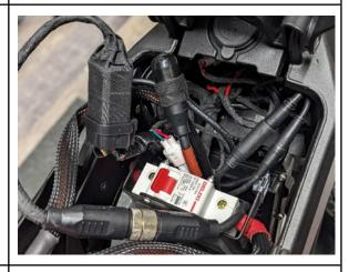
Step 17: Carefully arrange the connectors and Bluetooth module behind the breaker and then slowly move the battery support plate back. Take your time to make sure none of the wires are getting pinched. Once the plate will hinge back into place, reinstall the (2) bolts with a 5mm hex key. Be sure to leave out the battery connector and coms plug as shown in the picture. You can reinstall the ignition key plate and battery lid.
