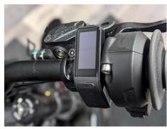
**Step 16:** Plug the 2 to 1 cable into the display and thumb throttle. Carefully route the 2 to 1 cable under the ignition plate and plug it into the X-9000. Plug in the Bluetooth and X-9000 adapter.
