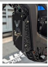
**Step 21:** Snug up the top controller bolts and check to make sure all the other bolts are tight. Reinstall the battery.
