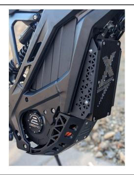
**Step 10:** Remove the battery lid and key switch plate with a 4mm hex key to provide access to the wires in the following steps.
