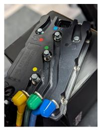
**Step 9:** Use the X-9000 box to support the X-9000 and a 5mm hex key to install the (3) phase wires.
