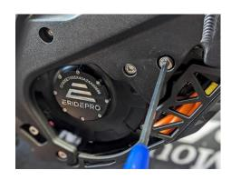
Step 4: Lower the front of the skid plate down.
