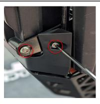
**Step 3:** Use a 5mm hex key to remove the (2) upper skid plate bolts.
