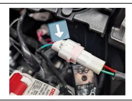
**Step 8:** Unbolt the (5) wires from the OEM controller using a 10mm socket. Unplug the main connector at the top.
