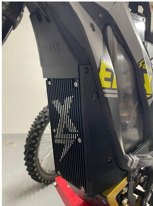
Figure 4: Attached side piece and upper piece shown. Printed from PLA-Basic on the Bambu Lab X1C
